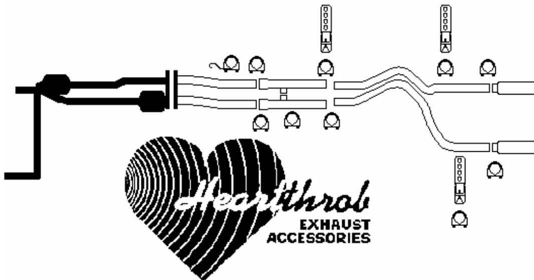
**NOTE:** do not tighten any clamps or nuts and bolts until the last step!! Before cutting any pipes it is a good idea to lay out all the included pipes along side the vehicle and get a good idea of how the pipes will hang on the vehicle. Please read the instructions fully and thoroughly before you begin
